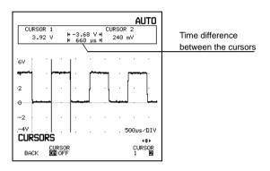
Cursor 1 is placed on the rising edge of the positive pulse, and cursor 2 on the falling edge.
