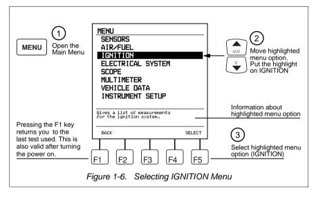
Subsequently follow steps (1) and (2) in Figure 1-7 to select SECONDARY IGNITION test.
