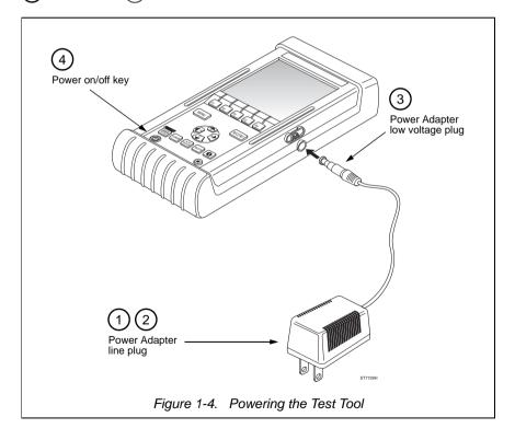
At power on, the test tool displays the model identification data. Press any key to display the vehicle data menu as shown in Figure 1-5.
