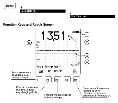
Figure 3-9. MULTIMETER VOLT display.
