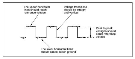
The duty cycle of the signal remains fixed, determined by the spacing between shutter blades.
