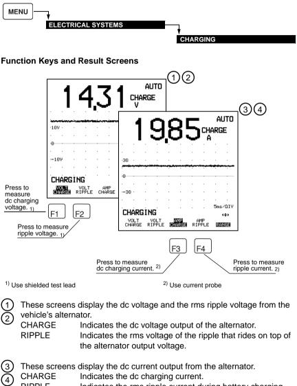
RIPPLE Indicates the rms ripple current during battery charging.
