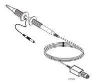
Used for RPM, injection pattern analysis, and advance tests on diesel engines with 6 mm fuel pipes. This set consists of a Piezo Pickup, which is clamped on the fuel pipe, a Probe-to-Piezo Pickup Adapter, a Low Pass Filter Probe to be connected to the test tool, and some additional accessories (not shown). Also see Appendix 7B under 'Optional Accessories'.
