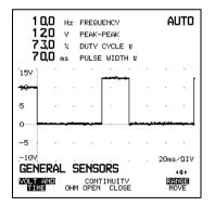
Figure 5-32. Result Display from a Mixture Control Solenoid Test
