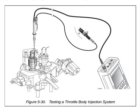
Current-Controlled (peak and Hold) Fuel Injector (Throttle Body and Port Fuel Injection Systems)
