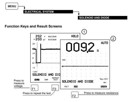
For the voltage test (F1 key), this is a single shot measurement, which means that the signal is displayed only once. To get a new test result, press the F3-key and reapply the signal from the solenoid.
