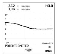
Figure 5-15. Result Display of a Voltage Test on a Ride Height Sensor
