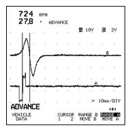
Figure 5-49. Result Display from an Advance Test
