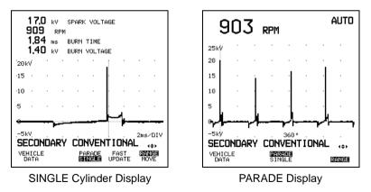
Figure 5-38. Result Display from Secondary Ignition Conventional
