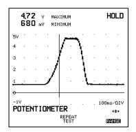
Figure 5-10. Result Display of a Voltage Test on a Potentiometer-Type Throttle Position Sensor
