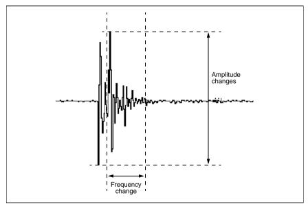
The pattern from this sensor is directly related to the cause and severity of the knock. For this reason each signal looks slightly different.
