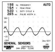
Figure 5-17. Result Display from a Magnetic Vehicle Speed Sensor Test
