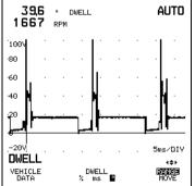
Figure 5-43. Result Display from a Dwell Test
