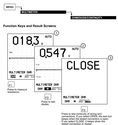
(1) This screen displays the measured resistance in ohms ( $\Omega$ ).
