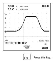
This is a single-shot measurement, which means that the signal from the potentiometer is displayed once. Turn the potentiometer slider from full counter clockwise to full clockwise or from full clockwise to full counter clockwise to get result display. To get a new test result, you have to press the F3-key and then turn the potentiometer again.
