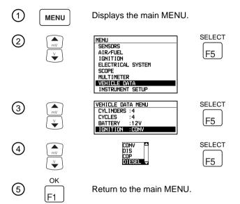
Proceed as follows to select the Diesel Injector test:
