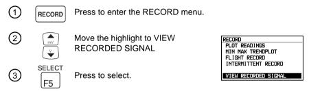
When you enter VIEW RECORDED SIGNAL, the display shows the readings that were on the display at the time you stopped recording. A vertical cursor appears at the location where these readings are valid, that is, at the end of the record. (See Figure 4-2)
