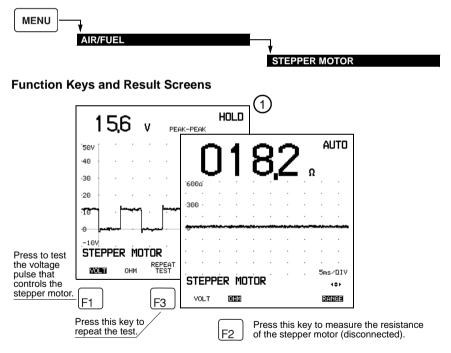
For the voltage test (F1 key), this is a single shot measurement, which means that the signal is displayed only once. To get a new test result, press the F3-key and reapply the signal from the stepper motor.
