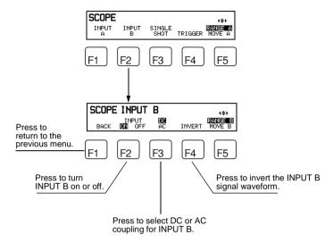
When you entered the scope function via the SINGLE INPUT SCOPE menu option, INPUT B is turned off by default, but you can turn it on by pressing F2. When INPUT B is turned on, GLITCH detection on INPUT A is turned off.
