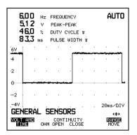
Figure 5-27. Result Display from an EGR Valve Test
