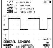
Figure 5-45. Result Display from a Hall Effect Distributor Triggering Test
