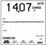
Figure 5-53. Result Display from Charging System Voltage Test
