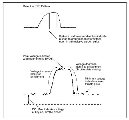
**Throttle Position Sensor (Potentiometer)**
