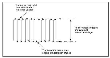
Voltage drop to ground should not exceed 400 mV.
