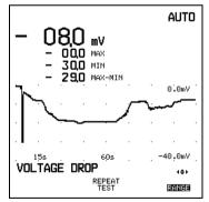
Figure 5-57. Result Display from a Voltage Drop Test
