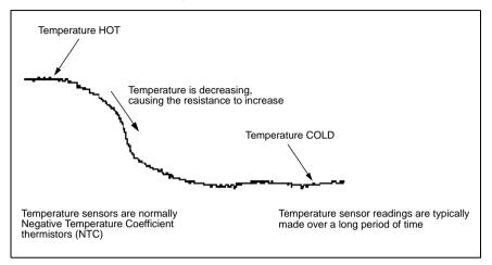
Coolant and Intake Air Temperature Sensors - NTC Thermistors
