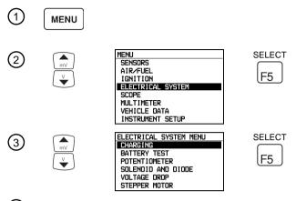
4 Connect the test leads as displayed by the test tool's Connection Help and shown in Figure 5-52.
