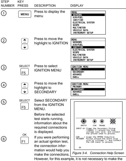
connections shown. Press F1 (OK) to actually enter the test.
