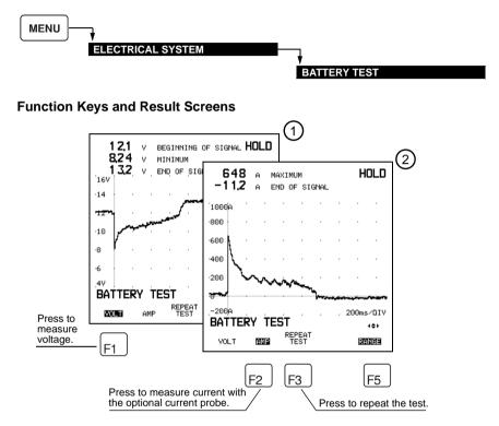
This test is a single shot measurement, which means that the signal is displayed only once. To get a new test result, stop the engine, press the F3-key and crank the engine again.
