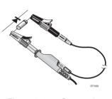
Figure 3-10. Connection for Diode Test.
