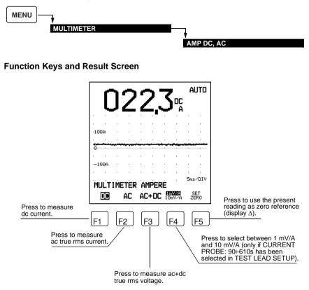
Figure 3-11. MULTIMETER AMPERE Display.
