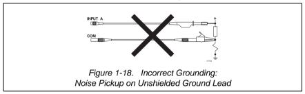
3. Measurement faults or short circuit with the DUAL INPUT SCOPE function. This occurs when you perform floating measurements with grounding at different points.
