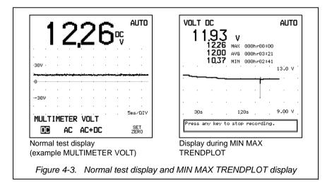
The graphical plot is displayed in the same way as PLOT READINGS, except in this function, time base rescaling does not stop after 16 minutes. Recording stops when you press any key on the Automotive ScopeMeter test tool.
