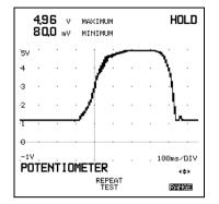
Use Potentiometer Sweep Test to test this volume Air Flow Meter (see page 5-15).
