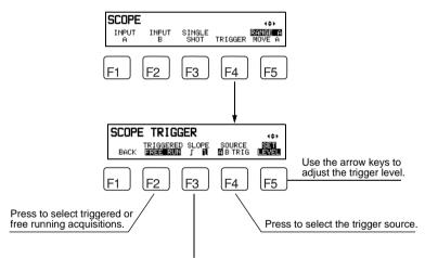
Press to select the trigger slope.
