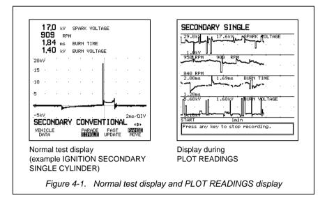
The plots that appear on the display are also written to memory for later examination. Memory contents are preserved when the test tool is turned off. (See the next section 'Viewing the stored results from PLOT READINGS'.)
