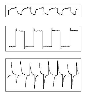
Idle Air Bypass waveforms may have unique shapes such as these and have a saw-curved appearance due to inductance reactance.
