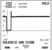
Figure 5-55. Result Display from a Solenoid and Clamping Diode Test
