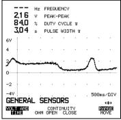
Figure 5-2. Result Display from a Map Sensor Test
