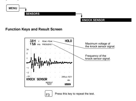
The test is a single shot measurement, which means that the signal from the knock sensor is displayed only once. To get a new test result, you have to press the F3-key and then tap the engine block or the sensor again. You may have to readjust the vertical range with the arrow keys to get an optimal waveform.
