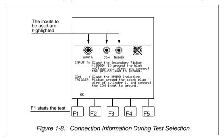
Press  $\begin{bmatrix} F1 \end{bmatrix}$  to start the test. For this example, it is not necessary to make the actual connections.
