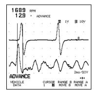
Figure 5-64. Advance at 1700 RPM.
